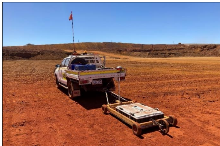
Ground Penetrating Radar testing for mapping voids beneath a mining pit floor, Pilbara WA.
