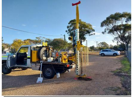
Photo 5. Test Location C1, Sub-surface Probing by Using a Drill Rig
