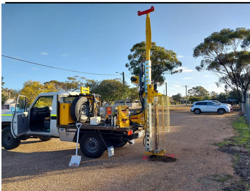
Photo 5. Test Location C1, Sub-surface Probing by Using a Drill Rig
