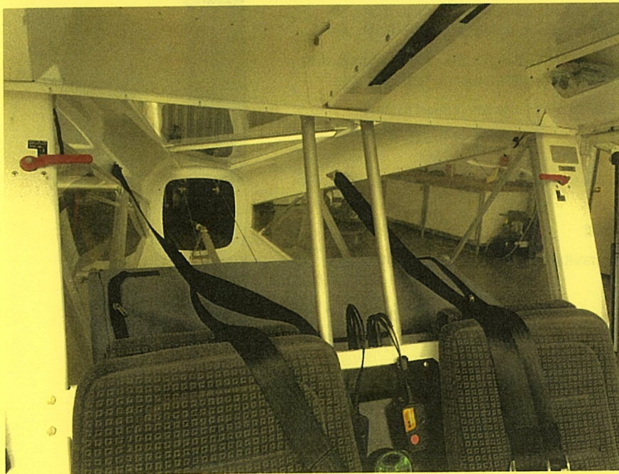
Fuel Shut-off valves
